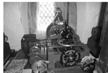
The Gillett & Johnston clock drives a vertical shaft which is connected by gears to the four clock faces.
