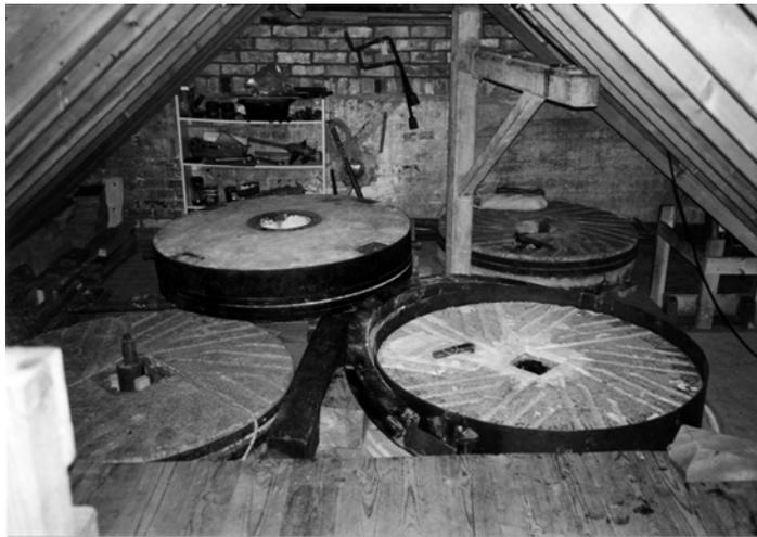
*The Stone Floor – showing the stone crane and 2 French Burr and 2 composite mill stones.*
